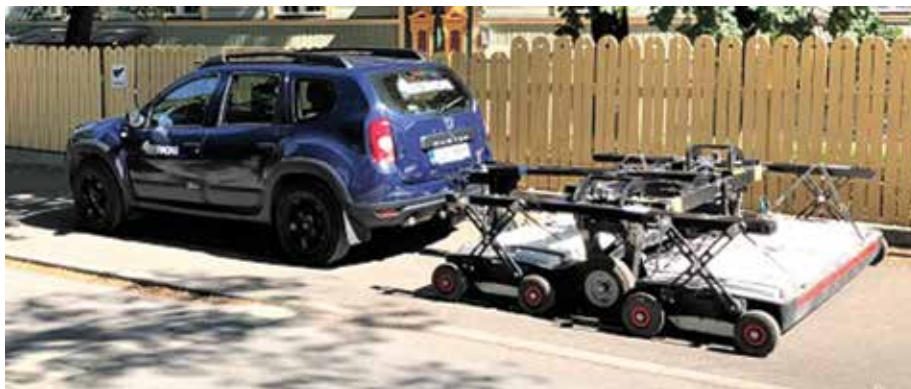
Picture 19: Testing the IDS Stream EM in Vesivärava Street
