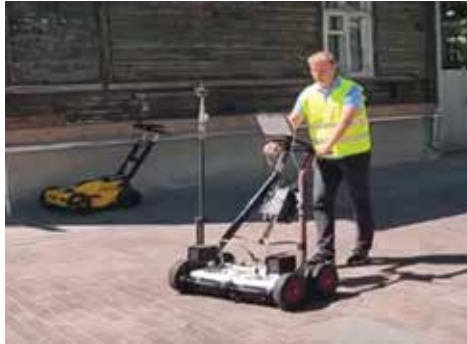
Picture 18: Olav Harjo participating in testing the IDS RIS MF Hi-Mod - in Vesivärava Street
