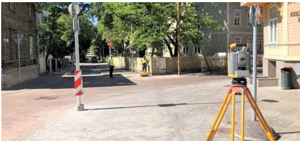
Picture 14: The crossing of Vesivärava, F. R. Faehlmanni and Wiedemanni streets with Total Station and IDS Opera Duo GPR
