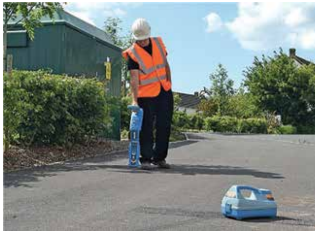
Picture 12: A survey using induction through ground (TSA, 2018) 18
