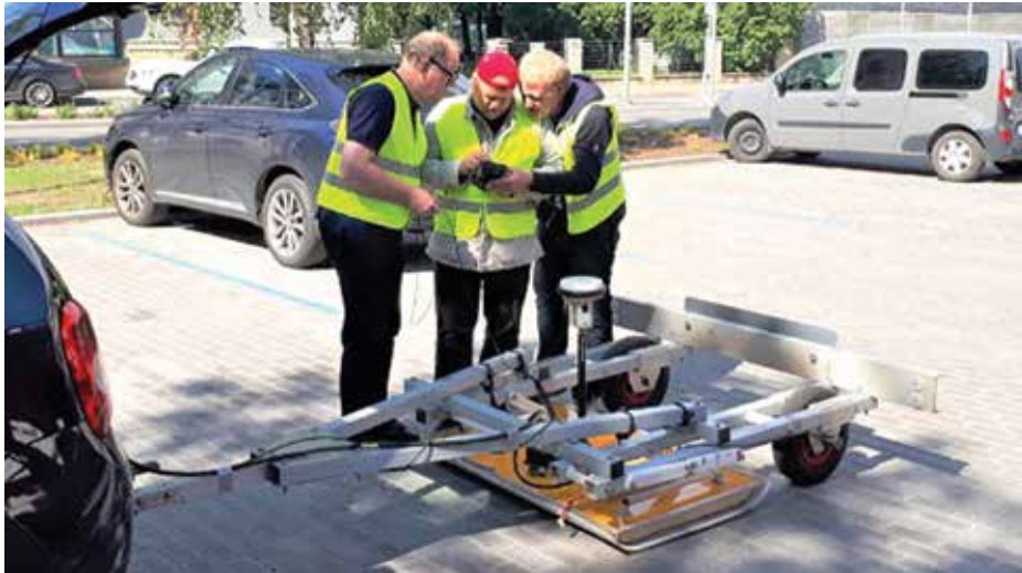
Picture 20: Emmanuel Thibaut, Andres Kärk and Raul Rokk participating in testing 3D-Radar GeoScope in Vesivärava street
