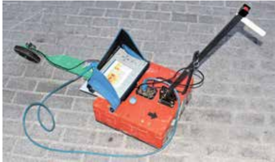
Picture 15: GPR GSSI SIR 3000 and 270 MHz antenna
